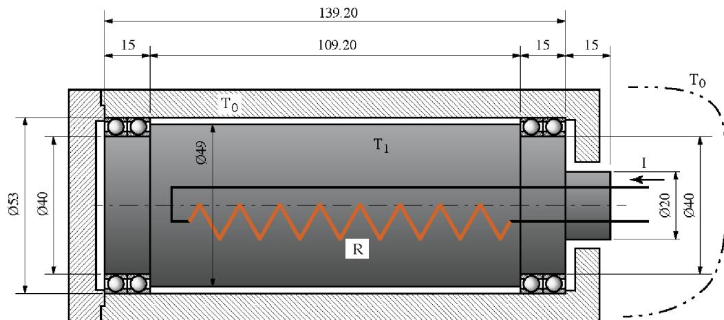
The temperatures of the axis ( $T_1$ ) and of the housing ( $T_0$ ) are considered to be homogeneous and in steady state equilibrium.
